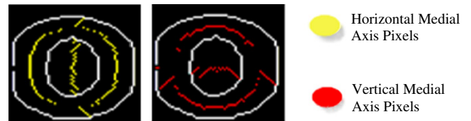
Fig. 6. Horizontal medial axis (left) and vertical medial axis (right).
