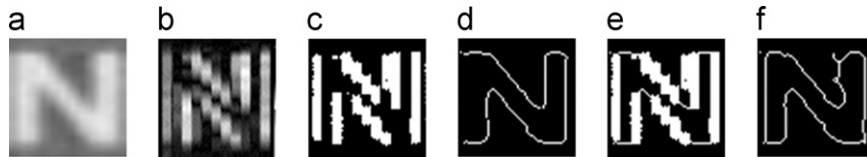
Fig. 4. Various steps of extracting character contours from grayscale input images. (a) Input, (b) NAG of (a), (c) text cluster of (b), (d) Canny of (a), (e) union of (c) and (d), and (f) thinning of (e).
