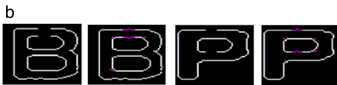
Fig. 7. Sample results of horizontal gap filling. (a) Illustration of horizontal gap filling based on VMP and (b) horizontal gaps filled. (For interpretation of the references to color in this figure caption, the reader is referred to the web version of this article.)
