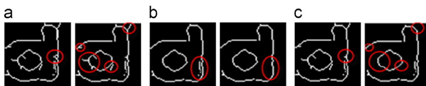
Fig. 11. Preprocessing steps during small gap filling. (a) Removal of small loops, (b) removal of small branches, and (c) removal of small blobs.
