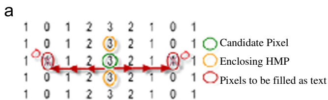
Fig. 7. Sample results of horizontal gap filling. (a) Illustration of horizontal gap filling based on VMP and (b) horizontal gaps filled. (For interpretation of the references to color in this figure caption, the reader is referred to the web version of this article.)
